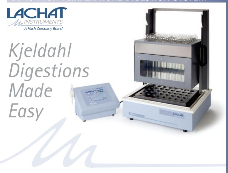
Lachat's BD40 Block Digestor will improve accuracy, precision and productivity of your high-temperature digestions. Developed to digest total Kjeldahl nitrogen and total phosphorus samples, the BD40 brings key features to this well-accepted block digestion technique.
